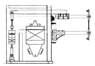
The main frame is high quality welded steel construction styled for trim appearance and functional design. The slim design requires a minimum of floor space. The upper arm extension is built integrally with the frame. The removable rear cover permits ready access to the frame interior for inspection and maintenance.
