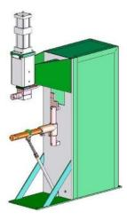
The main frame is high quality welded steel construction styled for trim appearance and functional design. The slim design requires a minimum of floor space. The upper arm extension is built integrally with the frame. The lower knee is steel, and supports the transformer; this allows the transformer to move up and down with the lower knee. A removable rear cover permits ready access to the frame interior for inspection and maintenance.
