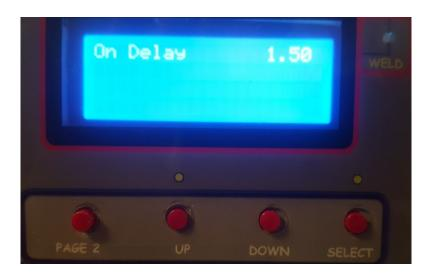
After programming the On delay (time befor relay is activated), use the SELECT button to advance to the next screen
