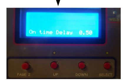
After programming the On Time Delay (time that the relay remains on), use the SELECT button to put the counter in run mode
