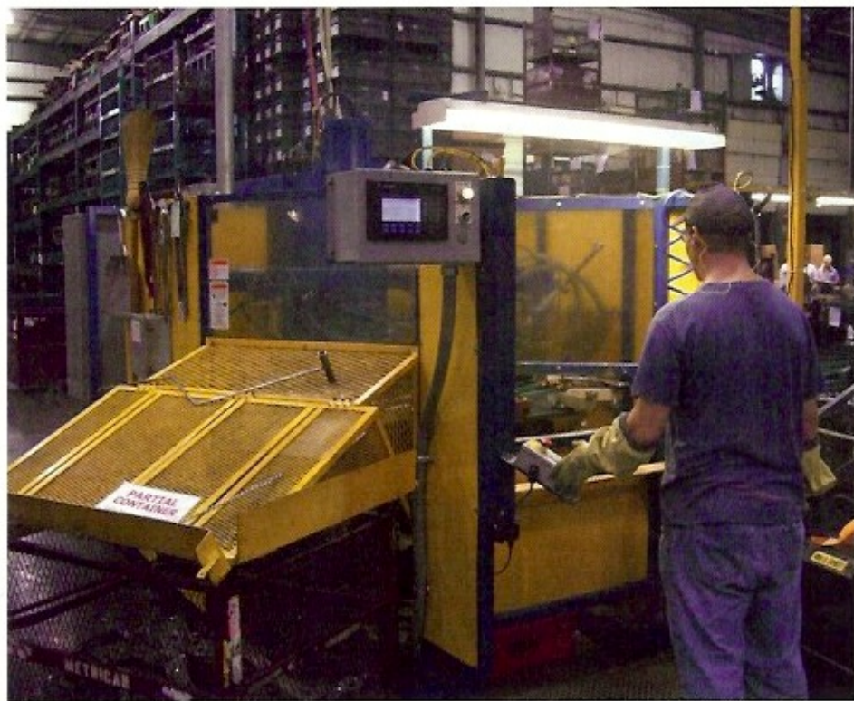
Metrican Stamping retrofitted this automated dial-index welding machine with MFDC technology, which delivers more energy to the welds and allowed the machine's cycle time to be reduced from 9.5 sec. to 7.5 sec., increasing production rate by 101 parts/hr.
