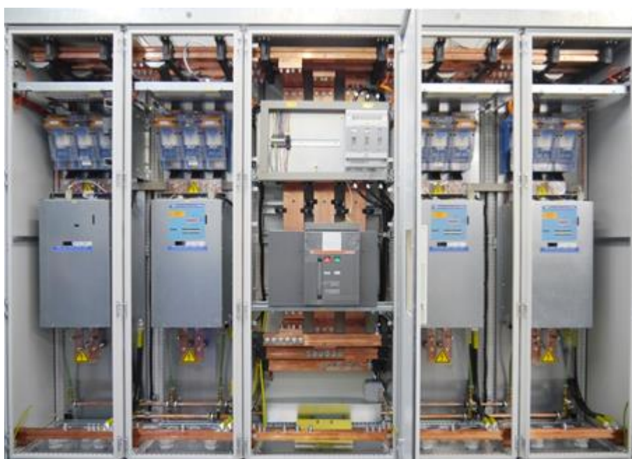
Fig. 6-3 Special system, maximum welding current 300 kA, SiniusHWI 3460 master system with three slave inverters
