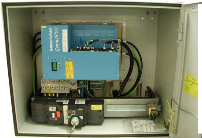
Fig. 10-1 Top mounted robot cabinet, interior view
