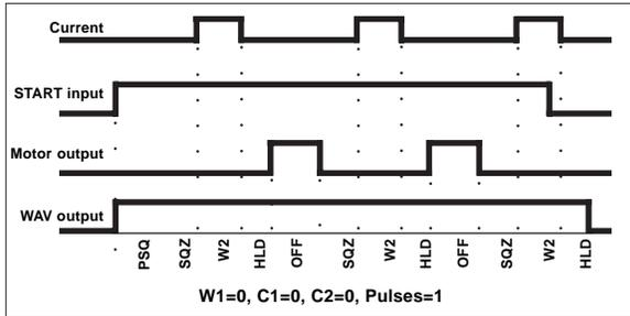
Figure 7-7. Roll-spot Welding
