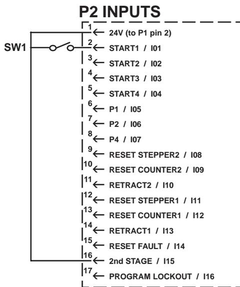
**Figure 9-1.** *Initiation switch connection*
