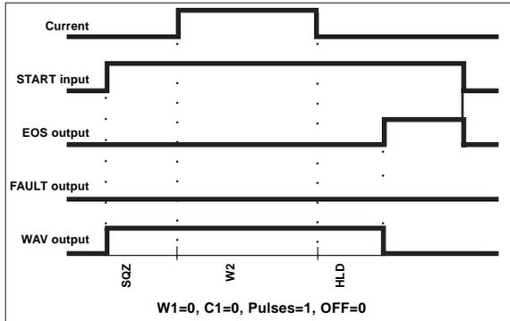
**Figure 7-1.** Basic Spot Weld—No Weld Faults
