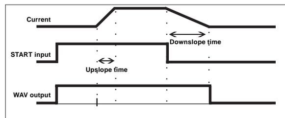
**Figure 7-6.** Seam Weld
