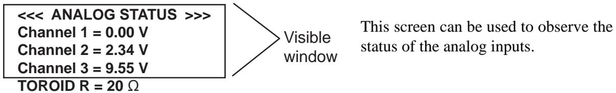
**Analog input channels 1, 2 and 3:** The dynamic voltage at each of the analog inputs. This is shown for test calibration purposes only and does not need to be adjusted by the user.
