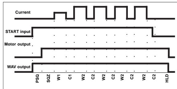
Figure 7-9. Seam Welding (Pre-heat)
