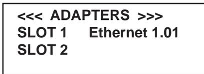
The EN1701 CPU can be configured with up to two adapter cards, to provide additional functions.
