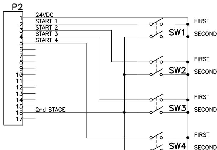
**Figure 5-3.** Multiple two-stage foot switches connection diagram
