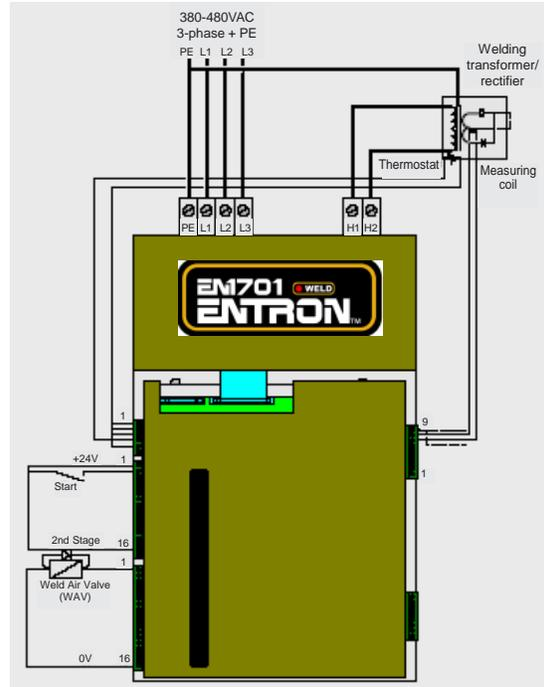
**Figure 5-4.** Basic connections
