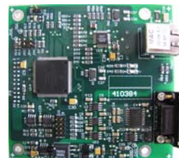
EIP/MBTCP Communication Card P/N 730014-013
