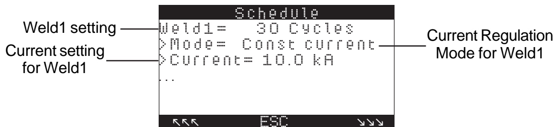
Figure 5-27. WELD1 in Constant Current mode
