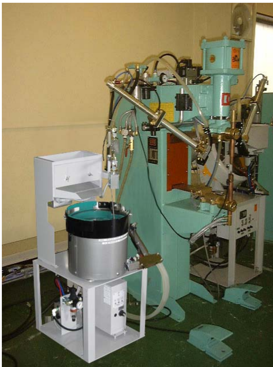
Automatic Nut Feeder combined with Spot welding machine
