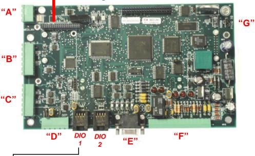
The "821" module connects to either DIO 1 or DIO 2 points of the "822" module. If you use two "821" modules then both DIO 1 & DIO 2 are used. The control automatically detects which module is connected to which port.
