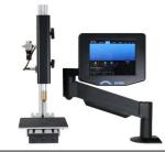
Orion 250i2 EV Arm Pkg. Orion Swing Arm Microscope, Orion stylus & all standard Orion 250i2 accessories.
